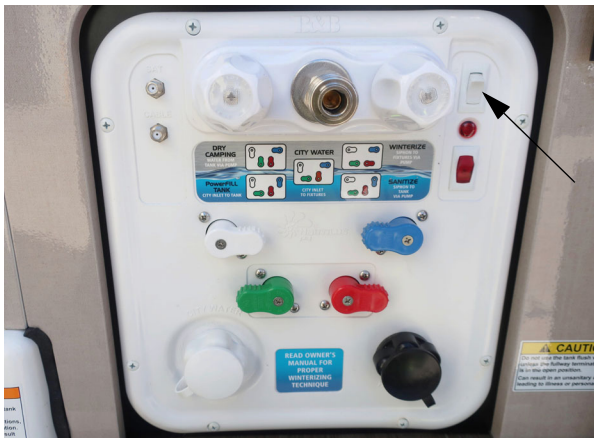
Water pump switch location on Water Center Panel *Model 59KL shown -Typical View
