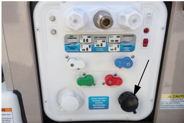
Black Waste Tank Flush Inlet (Located on Water Center Panel) -Typical View
