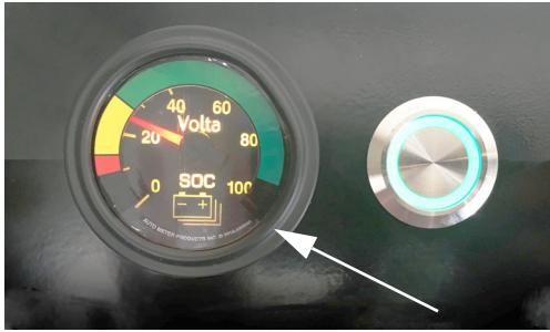
Pure 3 State of Charge (SOC) Gauge (Located on an interior cabinet) -Typical View
