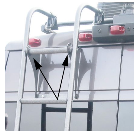
Ladder Storage Rungs -Typical View
