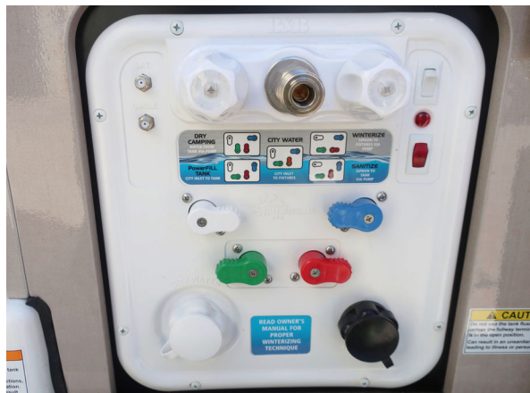
Water Center Panel in “Winterize” configuration (Panel located behind passenger rear door) *Model 59KL shown -Typical View
