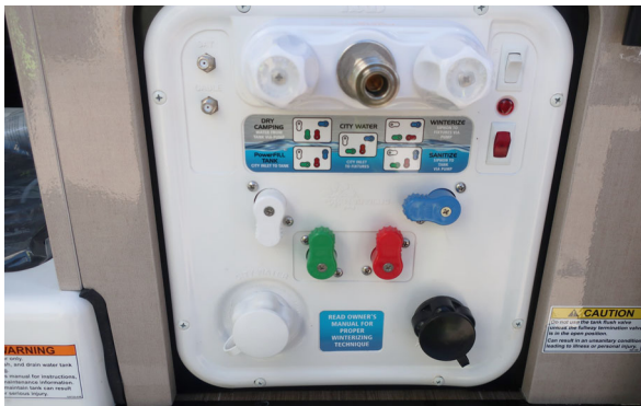
Exterior Shower/Wash Station (Located behind rear passenger side door on the 59KL, and behind the drivers rear door on the 59GL.) *Model 59KL shown - Typical View
