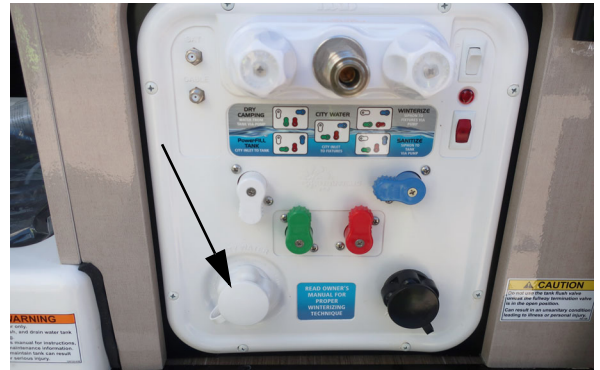
Tank Fill Inlet (Located behind the passenger rear door on the 59KL, and behind the drivers rear door on the 59GL.) *Model 59KL Shown -Typical View
