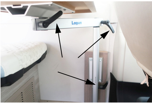
There are 3 adjustment levers that alter the height, length, and position of the table. -Typical View
