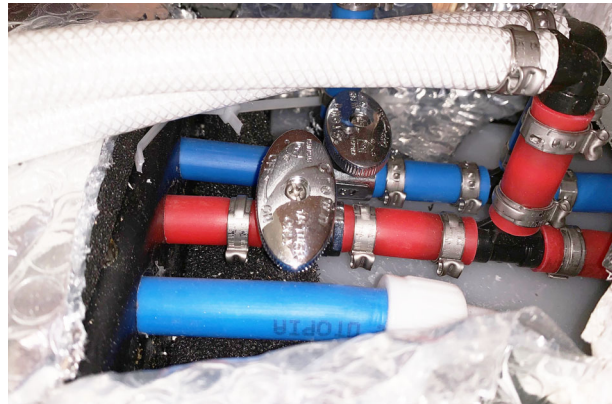
Waterlines and Tank Drain Valves *Model 59GL shown (See “Water System Drain Valve Locations” chart at the end of this section for location on your model) -Typical View
