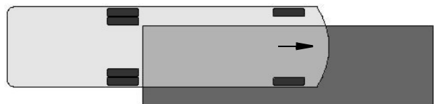
Weighing Right Front Corner
